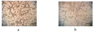
Fig. 2. A356 alloy microstructure before (a) and after treatment (b)
